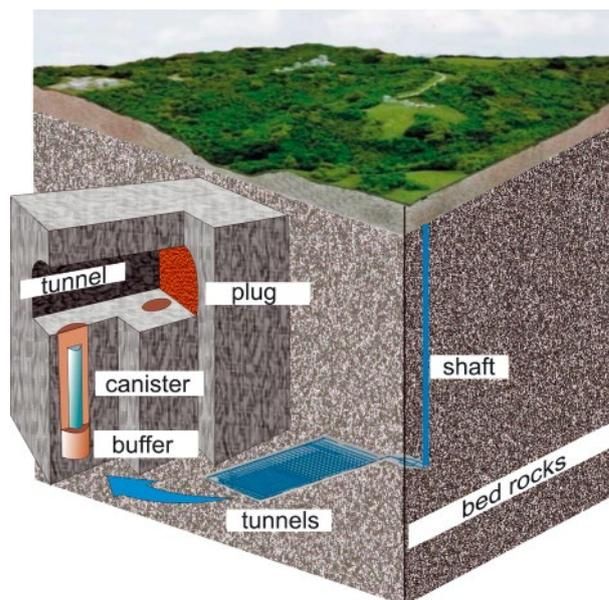
Figure 1. Layout of a multibarrier repository
