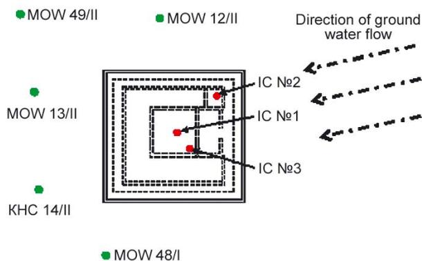
Figure 6. Layout of inspection channels (IC) inside RW SF EI-2; monitoring and observation wells (MOW) within the boundaries of RW SF EI-2 impact zone
