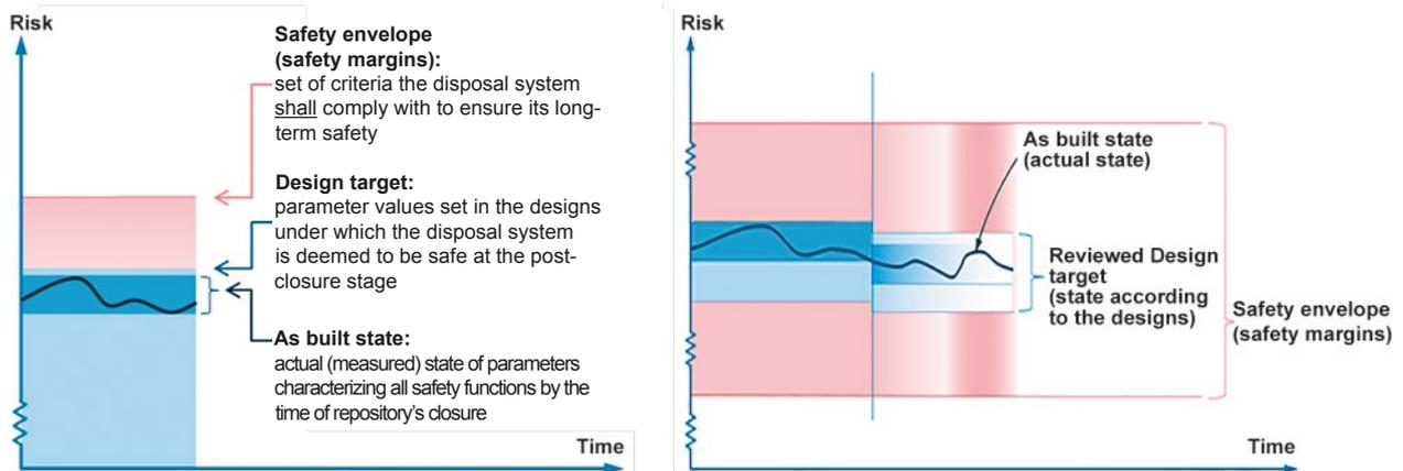
Figure 1. Visualization of Safety Envelope, Design Target and As Built State concepts (a) and example (b) of Design Target alterations due to Safety Case review
