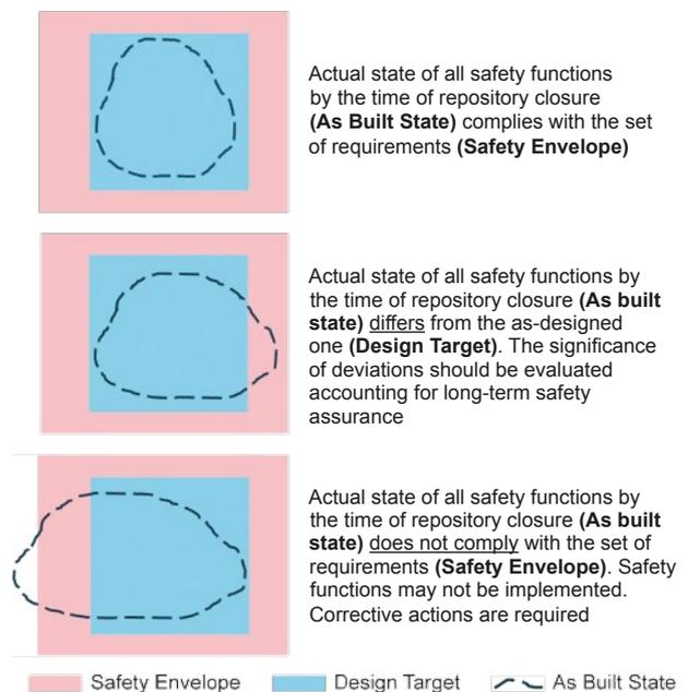
Figure 2. Cases presenting different relations between three states Safety Envelope, Design Target and As Built State
