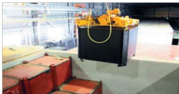
Figure 5. Emplacement of conditioned RW into a storage compartment
