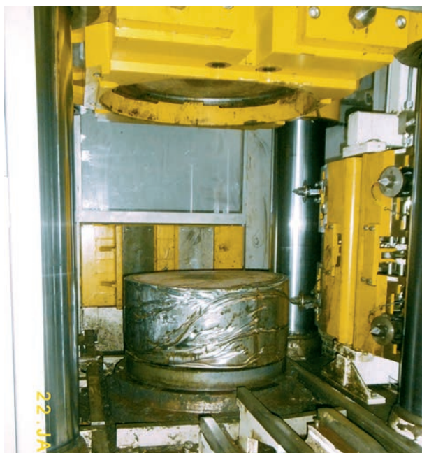
Figure 3. Drum filled with RW – before and after compaction
