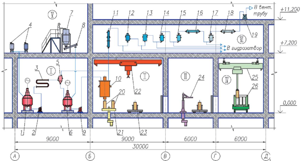
Figure 2. Hardware and engineering layout of a facility for BR vitrification at an NPP with WWER-1200 reactor units
