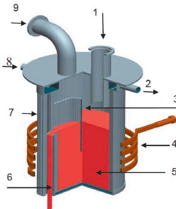
Figure 1. Induction melter with a "cold" type crucible
