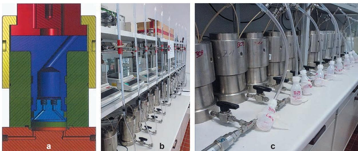
Figure 1. A construction drawing of the permeameter cell (a); supply of VGH to inlets at cell bottoms from burettes (b) to saturate bentonites and by a valve pump (c) to measure the permeability (regard plastic vessels connected to outlets at cell tops to collect percolating solutions)
