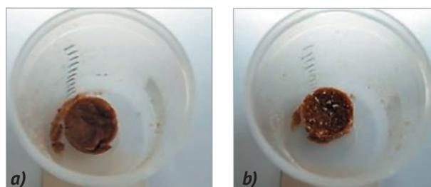
Figure 1. Samples after the solidification of bottom residue from evaporator: a) polymer No. 960 was used, the ratio of polymer mass to liquid mass (T:L) accounted for 1:5; b) a mixture of polymers was used (No. 960 – 90%, No. 910 – 10%), the ratio T:L = 1:5
