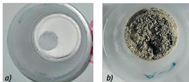
Figure 2. Samples after the solidification of solutions (polymer No. 960) with added silica (a) and zeolite (b); ratio T:L = 1:5
