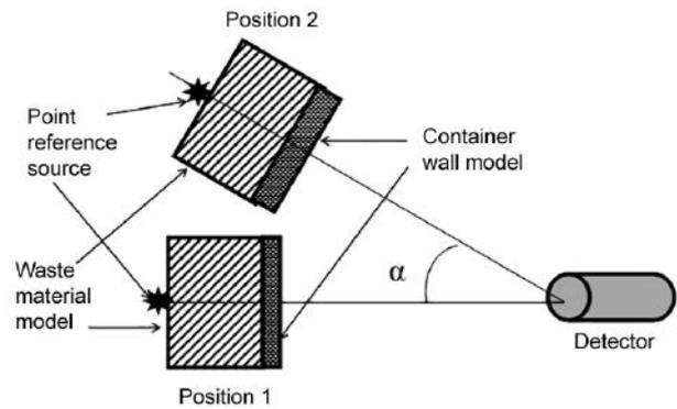
Figure 2. Model of a "point-source-behind-two-layers"
