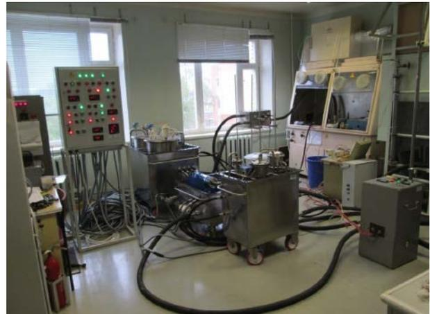
Figure 8. Modular unit for electrochemical decontamination (module box covers were removed)
