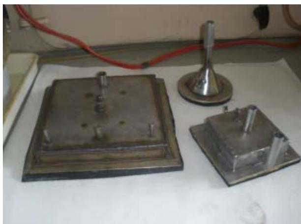
Figure 2. Stainless steel cells with an area of 0.4, 1 and 4.5 dm<sup>2</sup>
