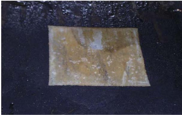
Figure 5. Flue section of RW incineration unit with an area of 1 dm<sup>2</sup> cleaned from soot and radionuclides using a mobile unit. Gas duct is made of stainless steel 12X18H10T
