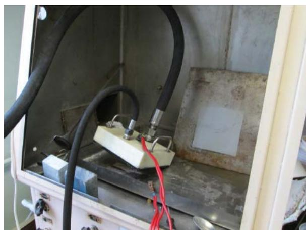
Figure 3. Cell with a 4 dm<sup>2</sup> caprolon body. In the background, a piece of metal decontaminated by this tool
