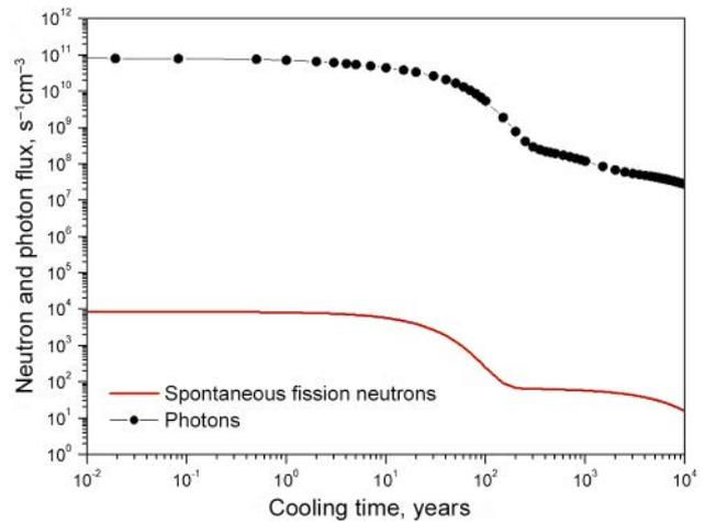
Figure 3. Cooling-time dependency of neutron and photon fluxes per BSS unit volume
