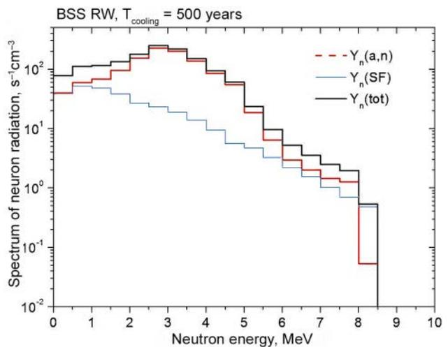
Figure 7. Energy spectrum of neutrons in vitrified RW and its constituent components due to spontaneous fission and  $(\alpha, n)$  reaction given a cooling time  $T_{cooling} = 500$  years
