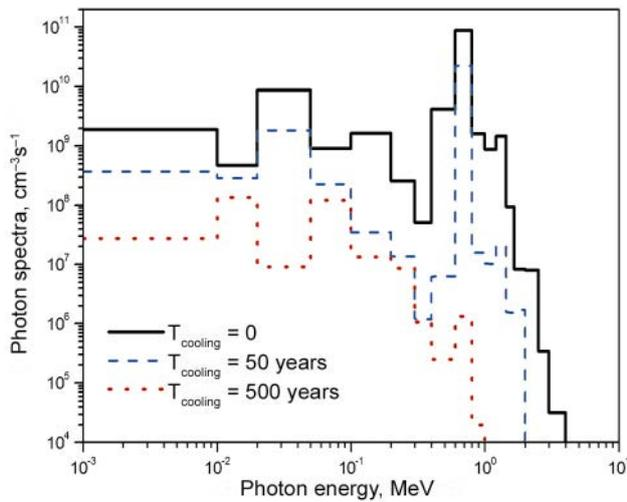
Figure 4. Energy spectrum of a bulk photon source considering different vitrified RW cooling times
