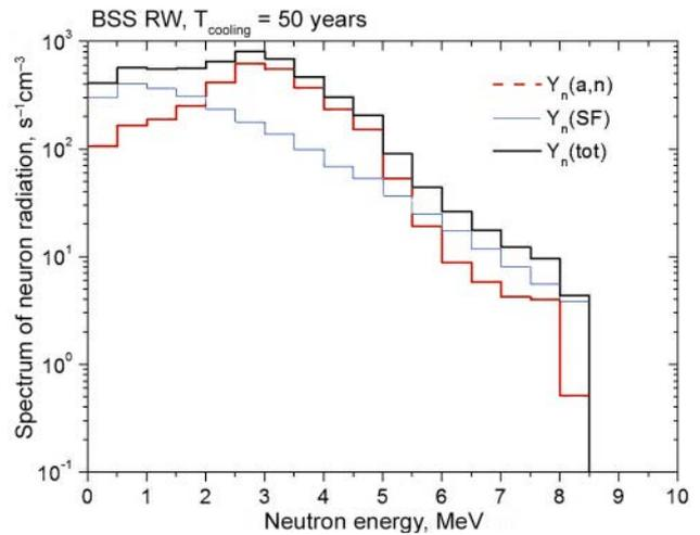
Figure 6. Energy spectrum of neutrons in vitrified RW and its constituent components due to spontaneous fission and  $(\alpha, n)$  reaction given a cooling time  $T_{cooling} = 50$  years
