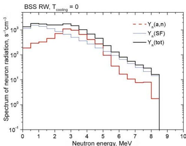
Figure 5. Energy spectrum of neutrons in vitrified RW and its constituent components due to spontaneous fission and  $(\alpha, n)$  reaction given a cooling time  $T_{cooling} = 0$  years
