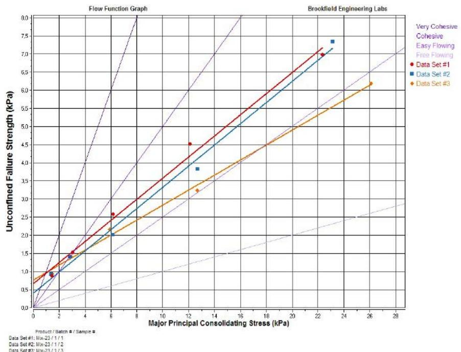
Figure 4. Brookfield PFTTM Dry Powder Flow Analyzer, blade cover for flow tests and measurement results for bentonite and kaolin mixtures with the following kaolin content: No. 1 – 50, No. 2 – 75, No. 3 – 85 wt. %
