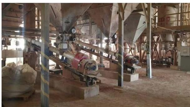
Figure 1. Production line for dispersed mixtures: GDE enrichment unit at the top, bins with emptying systems at the bottom
