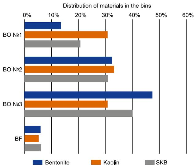
Figure 2. Mass distribution of materials in bins (BO) and bag filters (FR) in GDE tests under drying – grinding categorization mode
