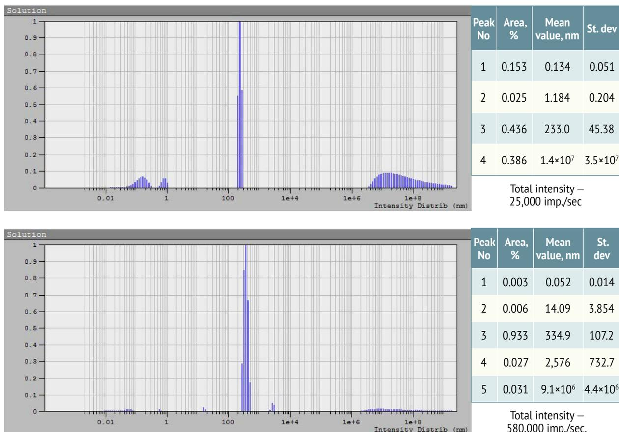
Figure 3. Particle size distribution in solutions following the interaction of model groundwater with Khakass bentonite without (above) and in the presence (below) of aluminophosphate glass at a temperature of 25 °C according to dynamic light scattering data
