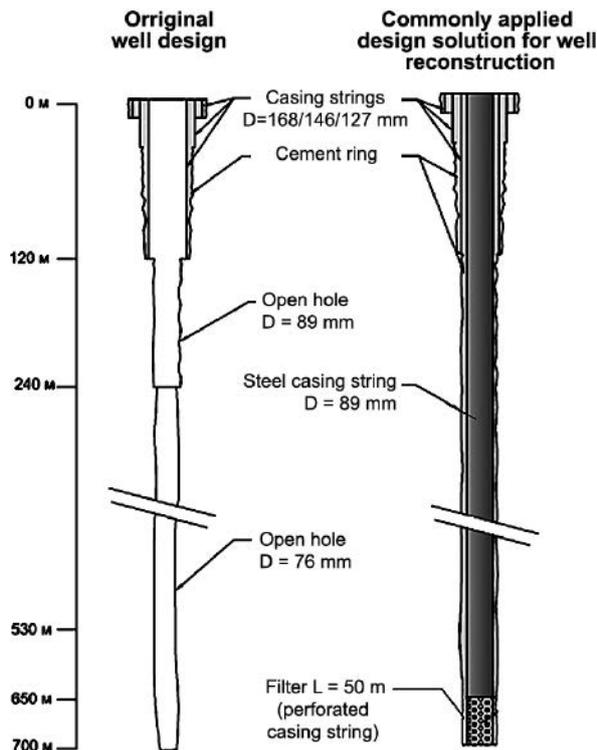
Figure 2. Snapshot of a commonly applied design solution for well reconstruction
