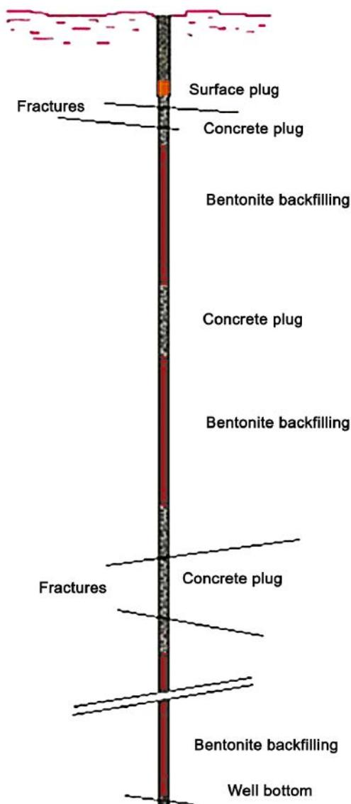
Figure 8. Schematic representation of the multi-layer plugging concept
