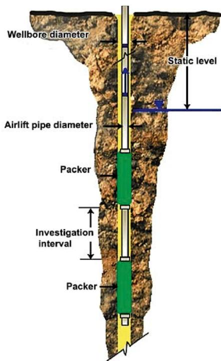
Figure 6. Option considered to arrange a two-packer system in an open section of a wellbore for interval monitoring purposes
