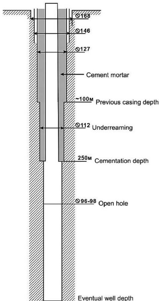
Figure 5. Well cementation at the Yeniseiskiy area
