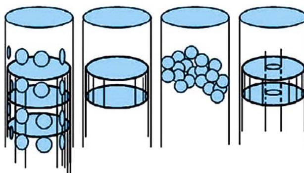
Figure 9. Advanced well abandonment technologies. From left to right: perforated tube, container method, pellets, stacking blocks
