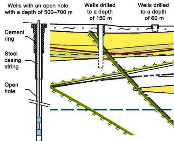
Figure 7. Examples of well designs planned for surface drilling in the Yeniseiskiy area
