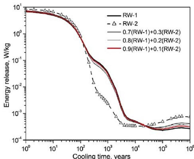
Figure 22. Relationship between the energy release and the cooling times for different vitrified RW compositions
