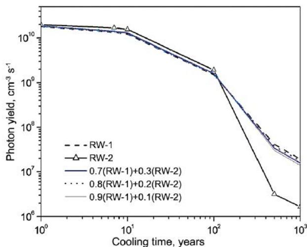
Figure 23. Relationship between the photon yields and the cooling times for different vitrified RW compositions
