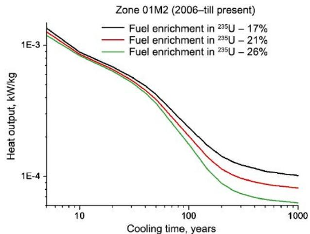
Figure 16. Change in SNF heat release for a fuel with different enrichment in  $^{235}\text{U}$  in zone 01M2 (2006–till present)
