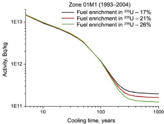
Figure 11. Changes in SNF activity for a fuel with different enrichment in  $^{235}\text{U}$  in zone 01M1 (1993–2004)
