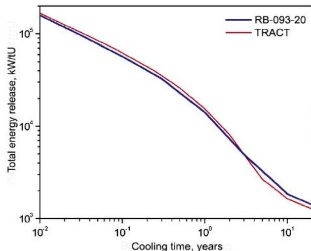
Figure 8. Change in the energy release of WWER-440 SNF with a fuel enrichment of 4.38% in  $^{235}\text{U}$  and a burnup of 36 GW-day/tU
