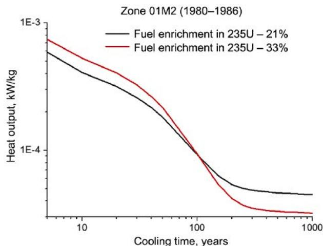
Figure 13. Change in SNF heat release for a fuel with different enrichment in  $^{235}\text{U}$  in zone 01 (1980–1986)
