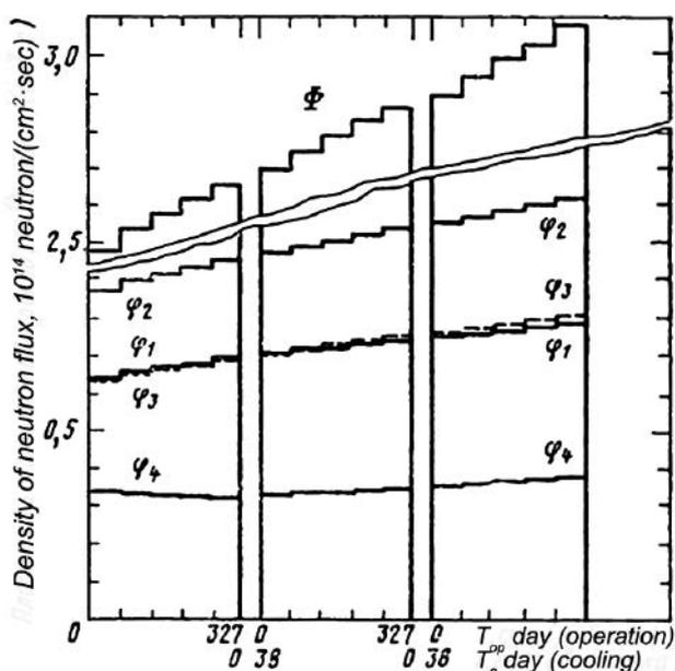
Figure 1. Irradiation mode for fuel (assemblies) with 3.6% enrichment at WWER-440 reactor unit
