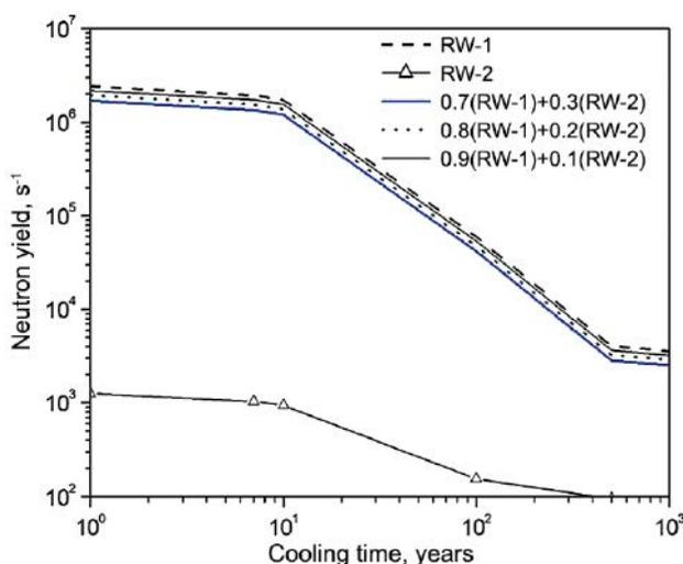
Figure 24. Relationship between the neutron yield and the cooling times for different vitrified RW compositions
