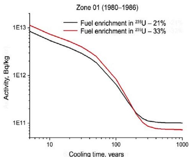
Figure 9. Changes in SNF activity for a fuel with various enrichment in  $^{235}\text{U}$  in zone 01 (1980–1986)
