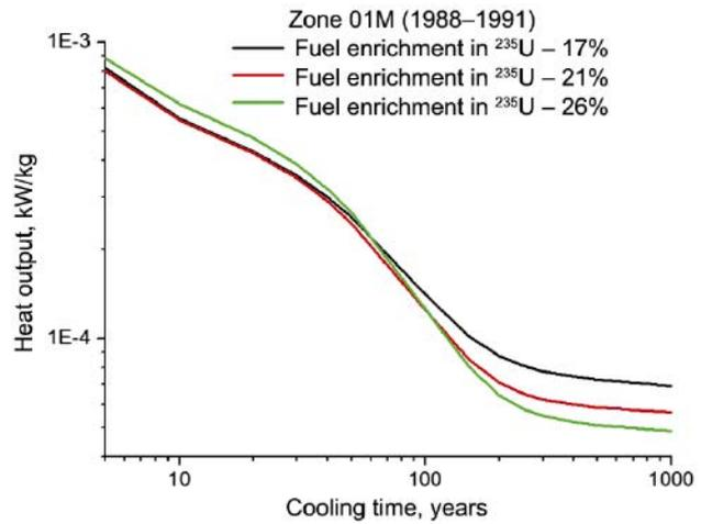
Figure 14. Changes in SNF heat release for a fuel with different enrichment in  $^{235}\text{U}$  in zone 01M (1988–1991)
