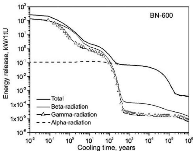
Figure 20. Energy release from SNF and its components associated with beta, gamma and alpha radiation from the BN-600 reactor
