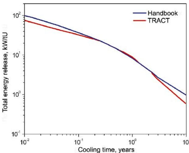
Figure 6. Total energy release from WWER-440 SNF
