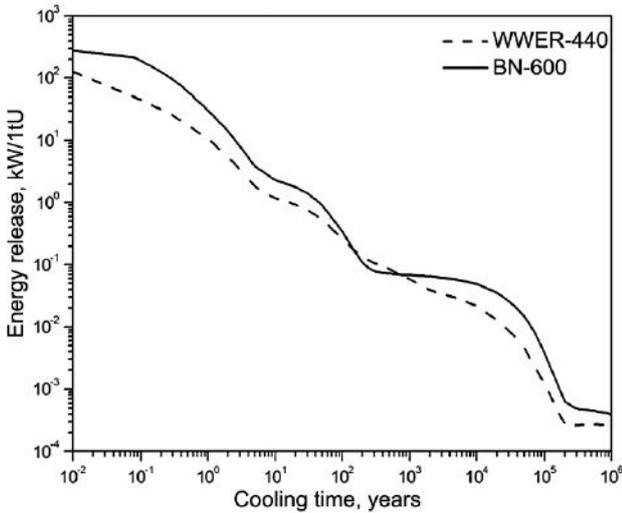
Figure 18. Energy release from WWER-440 and BN-600 SNF
