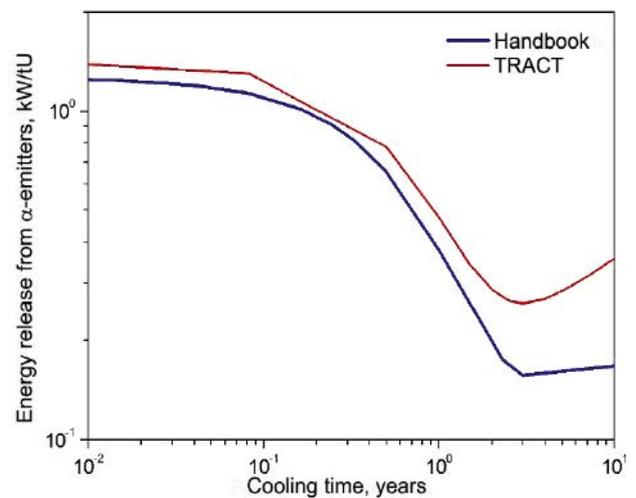
Figure 3. Changes in the energy release of alpha-emitters from WWER-440 SNF
