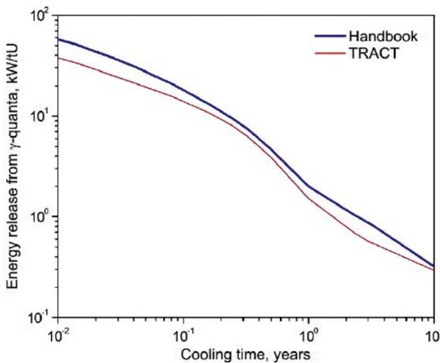
Figure 5. Changes in the energy release of gamma quanta from WWER-440 SNF
