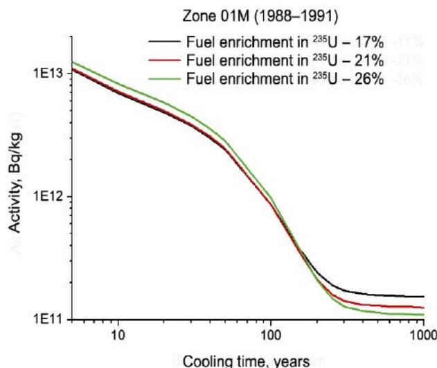
Figure 10. Change in SNF activity for a fuel with various enrichment in  $^{235}\text{U}$  in zone 01M (1988–1991)
