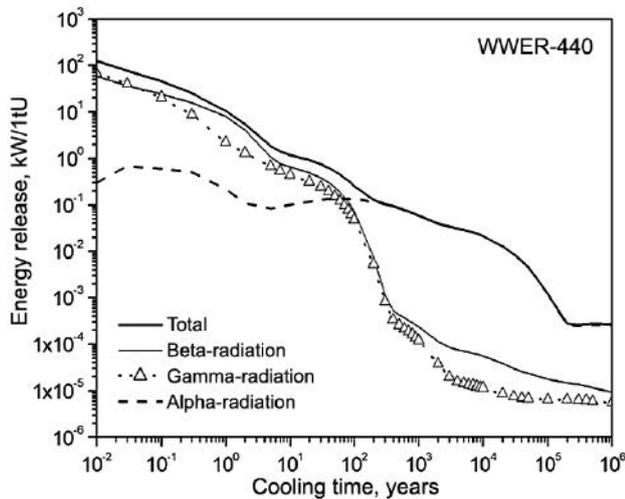
Figure 19. Energy release from WWER-440 SNF and its components associated with beta, gamma and alpha radiation from the WWER-440 reactor
