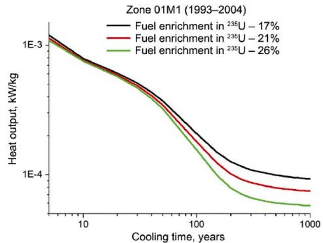
Figure 15. Change in SNF heat release for a fuel with different enrichment in  $^{235}\text{U}$  in zone 01M1 (1993–2004)
