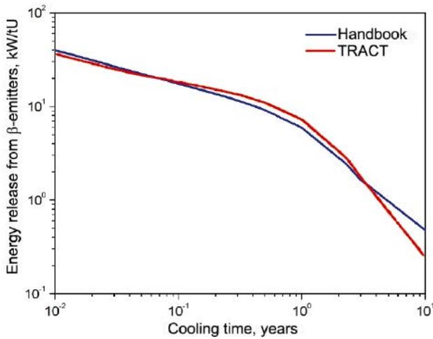
Figure 4. Changes in the energy release of beta-emitters from WWER-440 SNF
