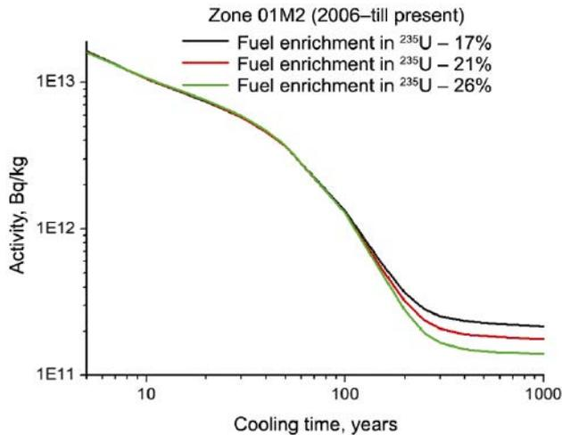
Figure 12. Change in SNF activity for a fuel with different enrichment in  $^{235}\text{U}$  in zone 01M2 (2006–till present)
