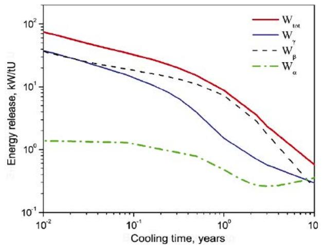
Figure 7. Total energy release from WWER-440 SNF and its constituent components
