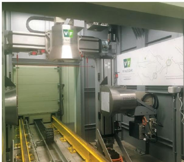
Figure 10. FRM-03, Chernobyl NPP, Ukraine. Measurement frame with semiconductor germanium detectors in a shielded tunnel made of low background material
