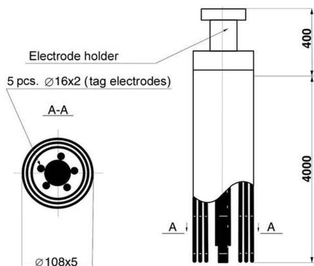
Figure 2. Rigged-up consumable electrode
