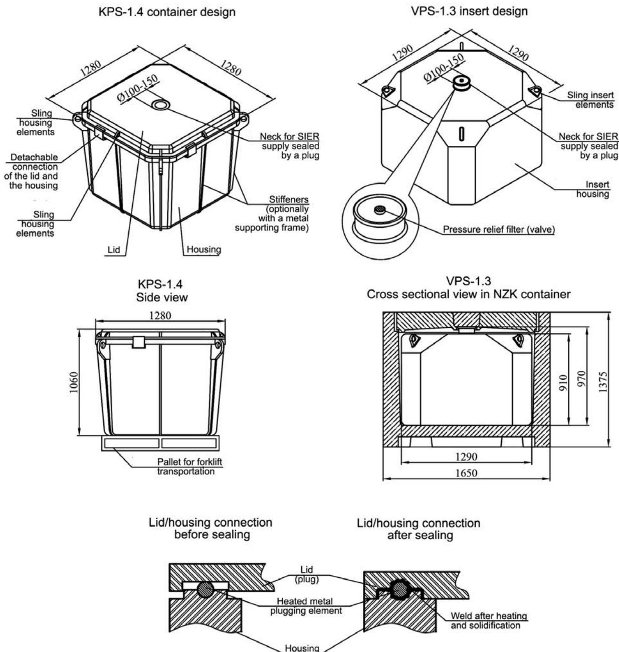
Figure 6. Designs of a polymer container for SIER Class 4 and VPS-1.3 polymer insert for the reinforced concrete NZK-150-1.5P container intended for SIER Class 3 packaging
