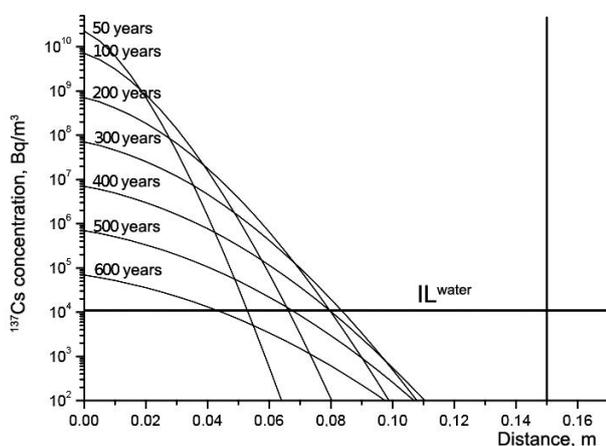
Figure 7.  $^{137}\text{Cs}$  concentration in the pore moisture of a container wall
