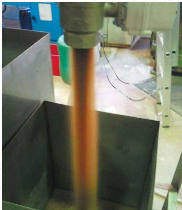
Figure 3. Pouring the dried product out of the resin dryer
