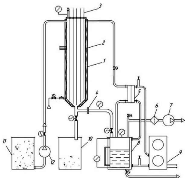
Figure 1. Process flow diagram for a SIER thermal vacuum drying unit:
