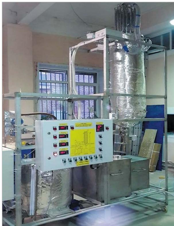
Figure 2. Pilot demonstration SIER drying unit
