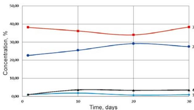
1 – portlandite on the sample surface; 2 – portlandite inside the sample (at a depth of 2 mm); 3 – calcite on the sample surface; 4 – calcite inside the sample (at a depth of 2 mm).
