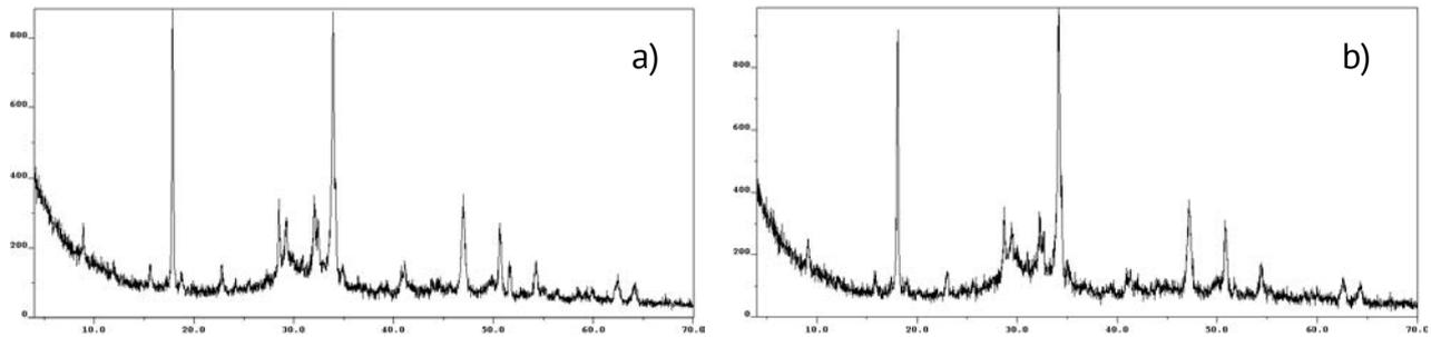
Figure 7. Registered diffraction patterns for a material layer of the PCT-I-G-50 sample at a depth of 2 mm given an exposure time of 10 (a) and 30 (b) days
