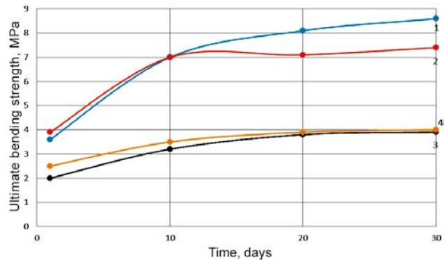
1 - backfill Portland cement at an exposure temperature of 20 °C; 2 - backfill Portland cement at an exposure temperature of 60 °C; 3 - 90:10 (%) cement-bentonite mixture at an exposure temperature of 20 °C; 4 - 90:10 (%) cement-bentonite mixture at an exposure temperature of 60 °C
