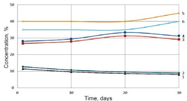
1 – alite in a cement-benotnite mixture (90%:10%) sample; 2 – alite in a backfill Portland cement sample; 3 – portlandite in a cement-benotnite mixture sample (90%:10%); 4 – Portlandite in a backfill Portland cement sample; 5 – amorphous phase in a cement-benotnite mixture sample (90%:10%); 6 – amorphous phase in a backfill Portland cement sample.
