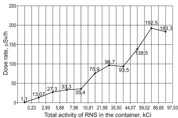
Fig. 4. Maximum gamma-radiation dose rate at the side surface of the package as a function of loaded activity
