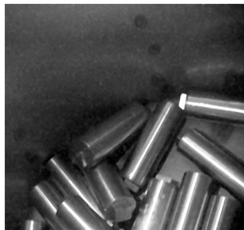
Fig. 8. SSRS inside the KMZ-RNI-RADON vessel
