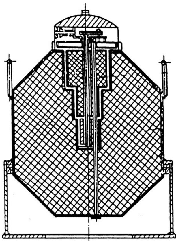
Fig. 1. Design of KTB-26-12 sources transportation container
