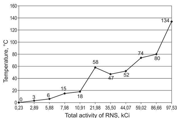
Fig. 3. Diagram of temperature change in the source vessel as a function of activity of loaded Co-60 sources
