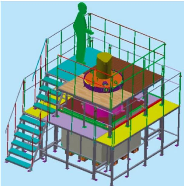
Fig. 6. Additional pad with railing of the conditioning kit
