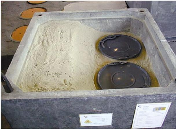
Figure 1. RW disposal package with NZK-150-1.5P container
