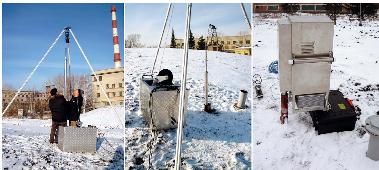
Figure 9. Assembling and setting up the neutron-gamma logging complex (left); implementing neutron-gamma logging via an inspection channel at RW SF EI-2 (center); implementing neutron-neutron logging using an inspection channel at RW SF EI-2 (right)
