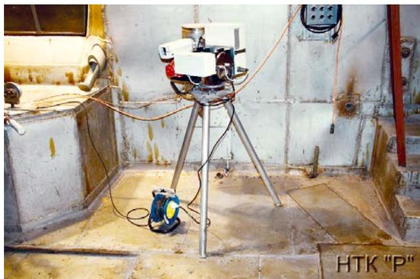
Figure 5. Gamma locator for individual SFA spectrometry survey
