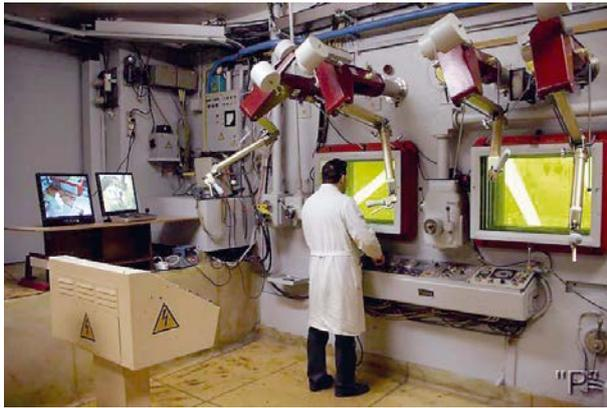
Figure 3. Console of the hot cell equipped with manipulators
