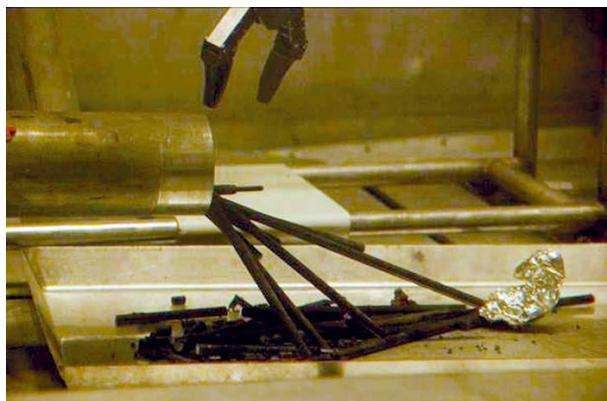
Figure 4. Fuel rods repackaging inside the hot cell
