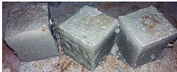
Figure 4. Cement compound samples manufactured from bottom residues with a residue/cement ratio of 1.5
