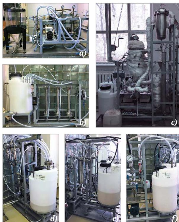
Figure 2. Layout of the laboratory bench for centrate treatment testing: pre-treatment unit (a), ion-exchange post-treatment unit (b), evaporation and drying unit (c), three-stages of condensate purification unit using the reverse osmosis method (d, e, f)
