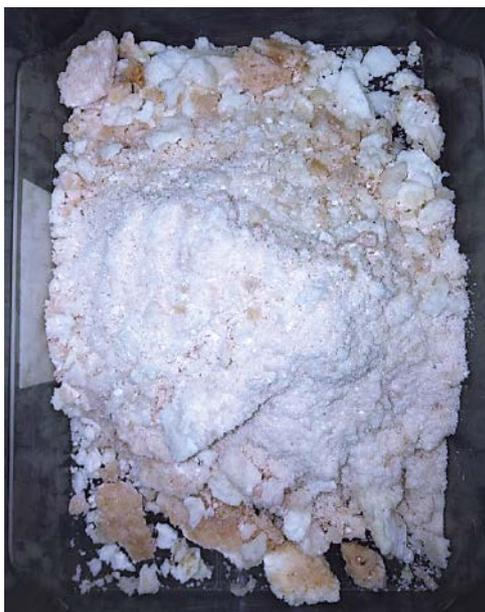
Figure 3. Dry salt residue of the centrate obtained at the stage of bottoms residue immobilization by drying
