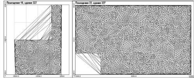
Figure 5. Example of a triangular mesh for L-shaped premises
