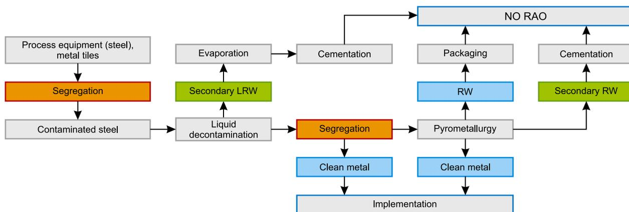
Figure 8. Operation flowchart for metal waste management (equipment and tiles)
