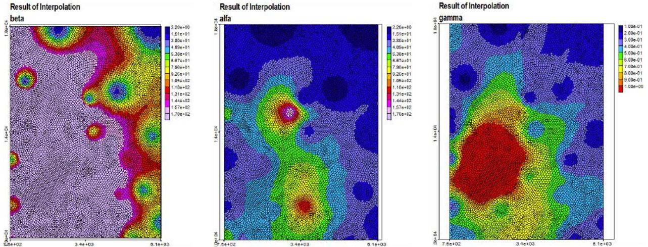
Figure 6. Cartogram of floor contamination with  $\alpha$ - and  $\beta$ -emitters and DER
