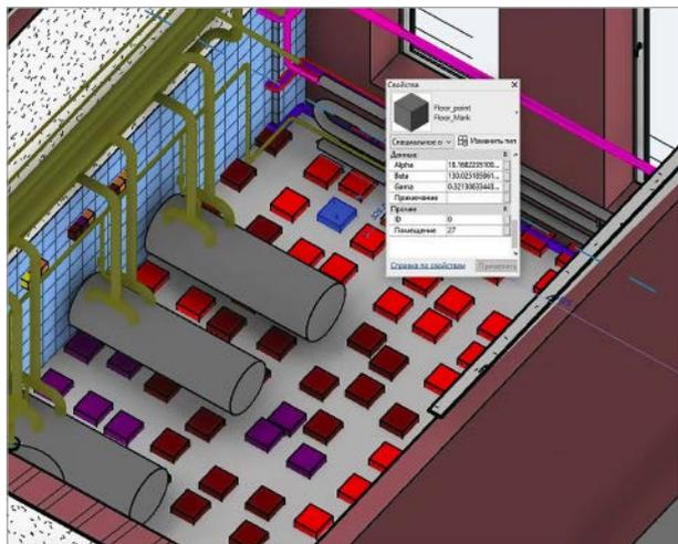
Figure 3. Model representation showing the measurement points for radioactive contamination on the floor
