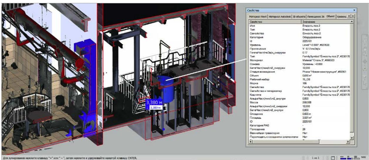
Figure 2. Level of geometry for key facilities considered important for the decommissioning exemplified by a BIM developed for building 327
