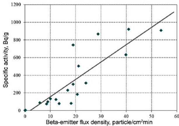
Figure 9. Dependence of specific activity on the flux density of beta-emitters from the concrete surface
