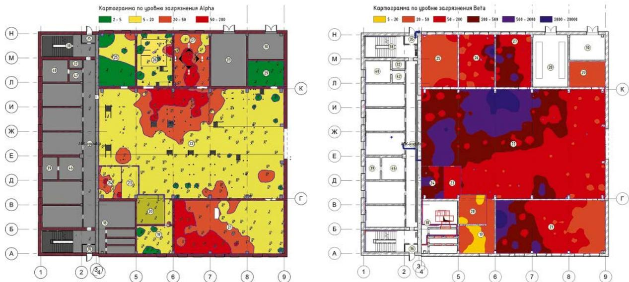
Figure 7. Cartograms of flux density considering  $\alpha$ -emitters (left) and  $\beta$ -emitters (right)
