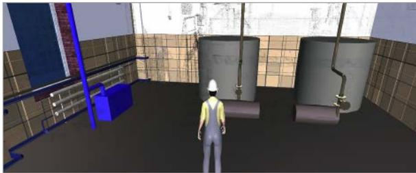
Figure 1. Information model. Level of geometry for the process equipment
