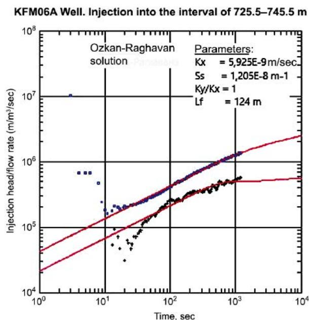
Figure 9. Results of vertical fracture injection interpretation. Blue dots — time tracking, black dots — diagnostic graph
