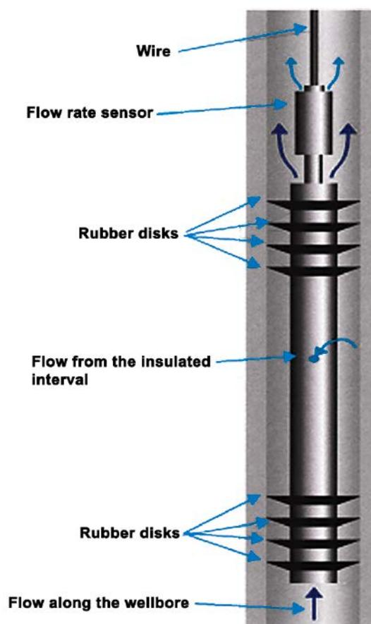
Figure 2. Differential flow measurement device
