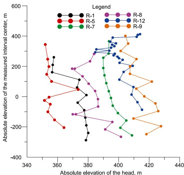
Figure 1. Distribution of heads along the depth in the wells of the Yeniseiskiy site
