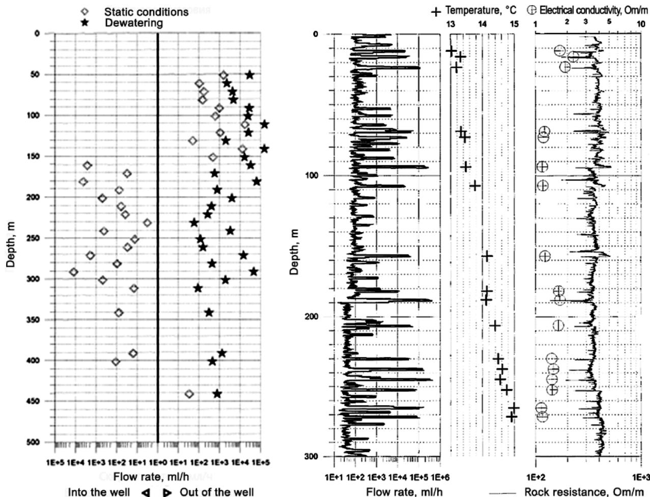
Figure 3. Results from the differential flow metering
