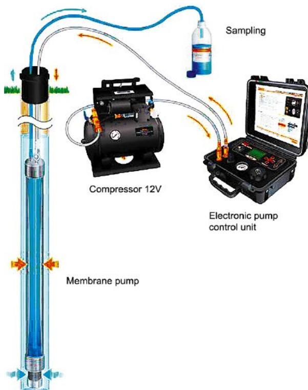
Figure 10. General layout of the diaphragm pump and its control elements
