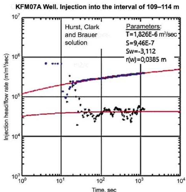
Figure 7. Interpretation of results considering the case of injection into an isolated fractured interval using the AQTESOLV software. Blue dots – time tracking, black dots – diagnostic graph
