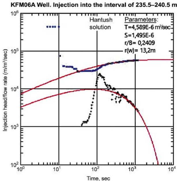
Figure 8. Interpretation of results considering the case of an injection into a fractured interval connected with an adjacent one. Hantush's scheme. Blue dots — time tracking, black dots — diagnostic graph
