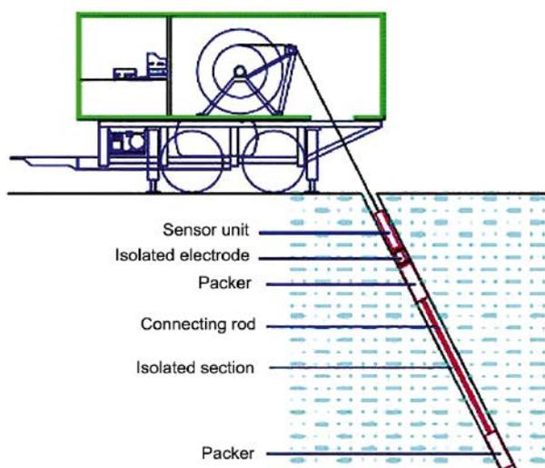
Figure 4. HTU equipment for interval injection
