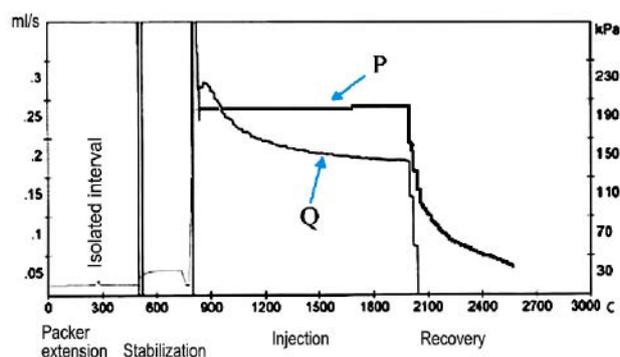
Figure 5. Typical injection curve for a constant pressure interval
