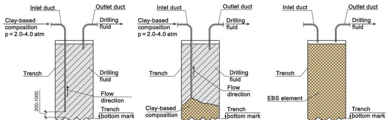
Figure 1. Impervious curtain of a "buried wall" type based on BentInject composition
