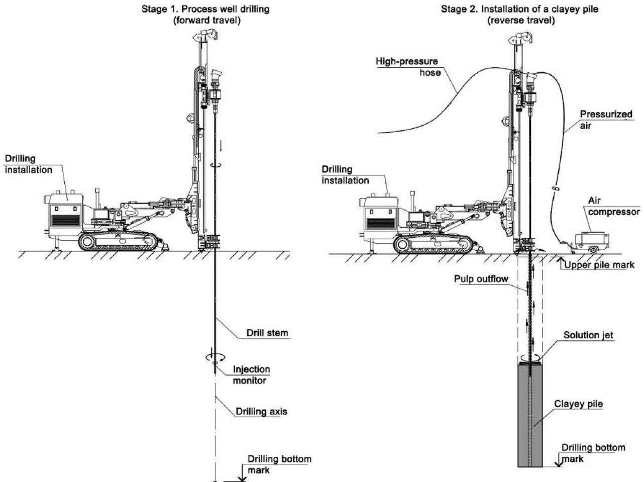
Figure 2. Layout of a soil-clay pile based on BentInject composition
