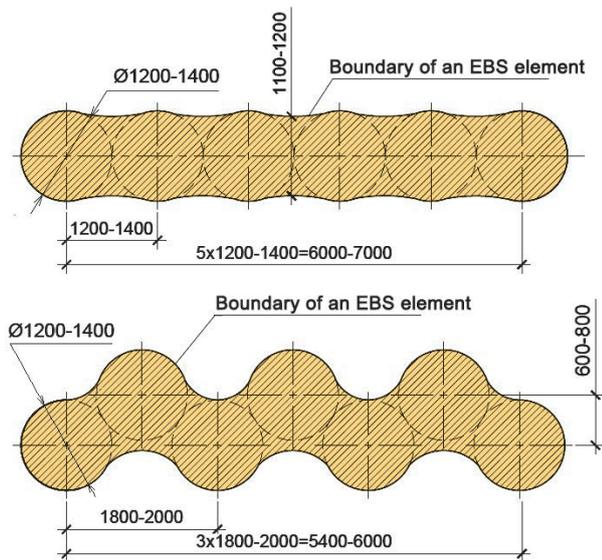
Figure 3. Different screen layouts involving clay piles (barrier elements)
