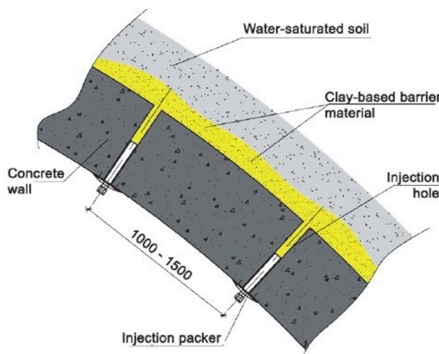
Figure 5. Layout of an insulation method involving contour injection based on BentInject composition
