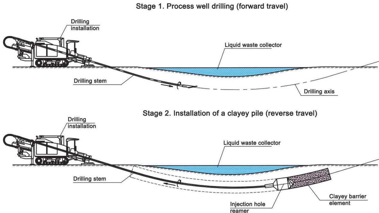
Figure 4. Stages of horizontal EBS clay-based element installation using the BentInject composition
