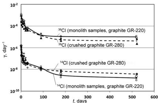
Figure 3. Dynamics of changes in the fraction of  $^{14}\text{C}$  and  $^{36}\text{Cl}$  leached out from the irradiated block graphite samples as per unit of time [14]
