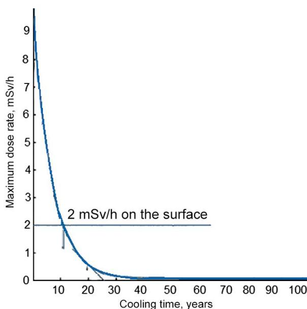
Figure 2. Equivalent dose rate from a graphite block depending on its cooling time
