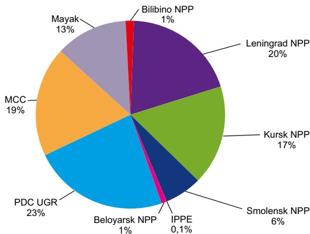
Figure 1. The inventory of irradiated graphite accumulated at different sites, as a % of the total mass [2]
