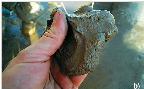
Figure 5. Paste filling based on uranium ore processing materials: a) supply through a pipeline, b) deep thickening paste
