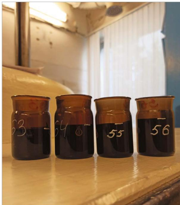
Figure 3. Appearance of BSC samples at an exposure dose of  $1 \cdot 10^6$  Gy
