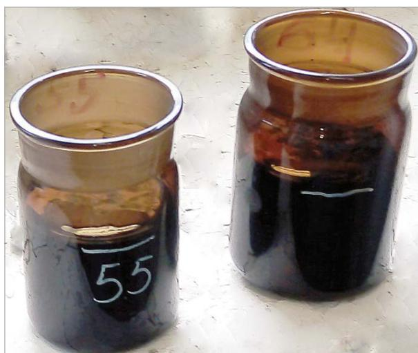
Figure 4. Appearance of BSC samples at an exposure dose of  $4 \cdot 10^6$  Gy
