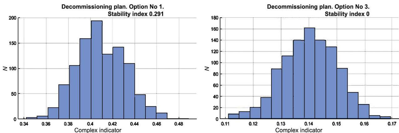
Figure 1. Stability calculations by the Monte Carlo method for options No. 1, 3 assuming equal priority coefficients of partial indicators
