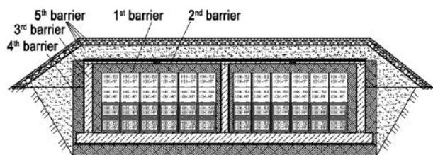
Figure 2. Near-surface disposal facility design developed for the sites of FSUE PA Mayak and JSC SCC [4]
