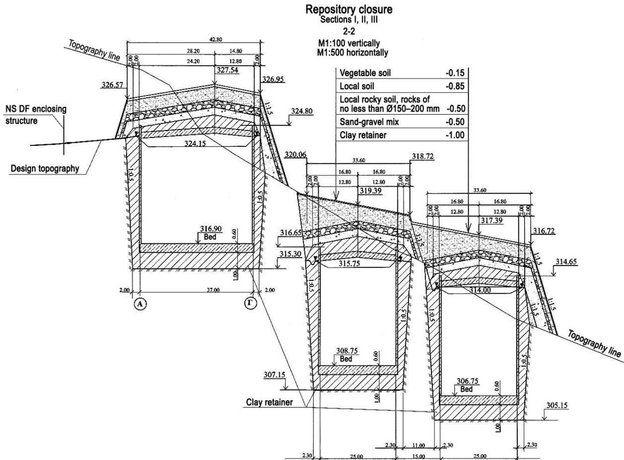
Figure 1. RWDF designs developed for the JSC UEIP site (containers and buffer material are not shown) [1]
