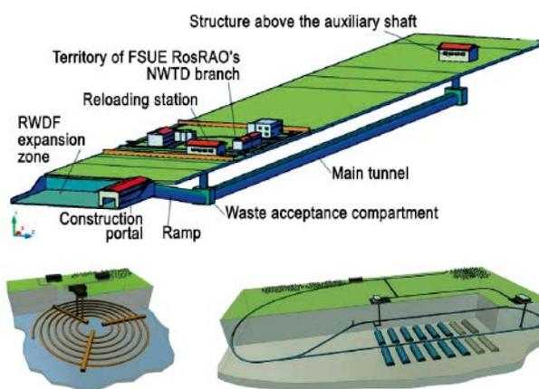
Figure 4. Examples of shallow designs for near-surface disposal facilities developed for the North-Western Territorial District of the Russian Federation: from above – a tunnel structure excavated using a tunnelling machine, at the bottom left – a spiral structure, at the bottom right – a chamber structure [25]
