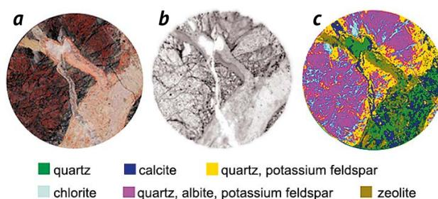
Figure 1. Distribution of cesium on the surface of the R-11 sample: a – optical image of the R-11 well sample, b – radiogram of cesium sorption on the R-11 sample, c – optical image of the R-11 well sample with mineral phases
