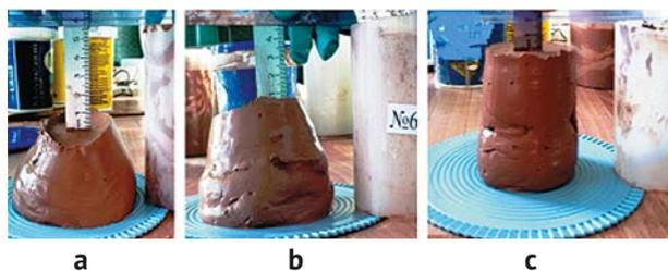
Figure 4. Rheological properties of the paste measured by the cone slump method given solids content of: a) 53%, b) 58%, c) 62%
