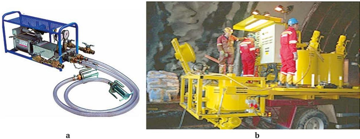
Figure 12. Engineering methods used to strengthen the rocks with polyurethane resins:
