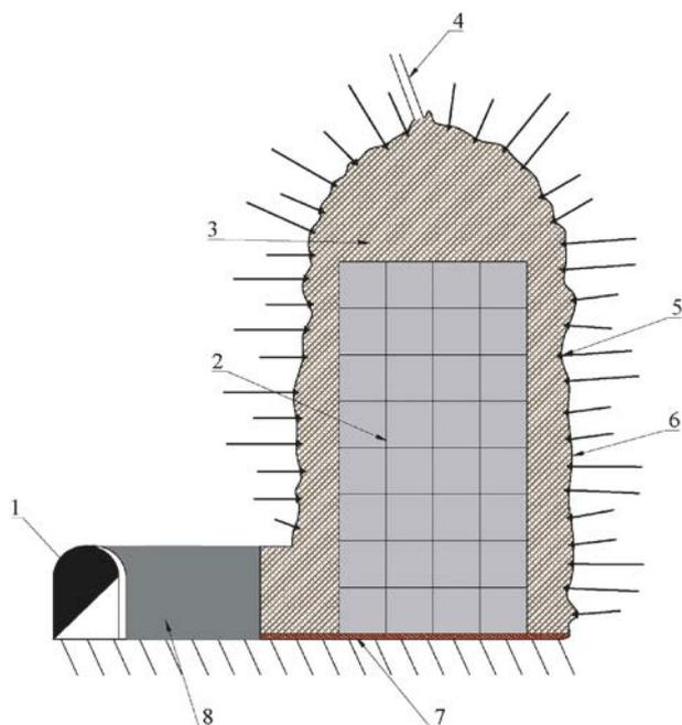
Figure 14. Disposal of containers with RW Class 2 and 3 in an abandoned chamber:
