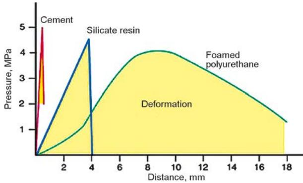
Figure 11. Comparison of strength (tensile) elastic properties of crack fillers during injection: cement, silicate resins, foaming polyurethanes
