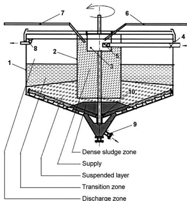
Figure 5. Layout of the thickener tank: 1 – thickener tank, 2 – flocculation chamber, 3 – mixing chamber, 4 – supply pipeline, 5 – tangential inlet to the mixing chamber, 6 – first-stage flocculant pipeline, 7 – second-stage flocculant pipeline, 8 – drain box, 9 – sludge discharge, 10 – sludge removal mechanism
