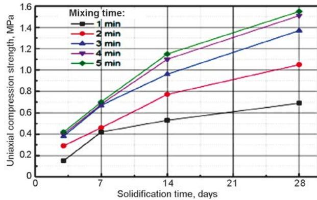
Figure 8. Dependences between the compression strength of a paste filling and the mixing time of the components
