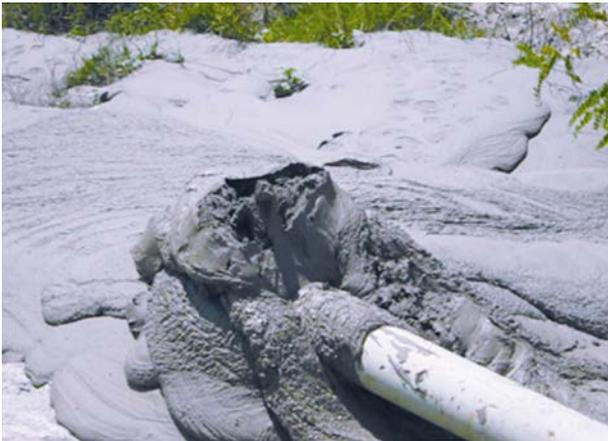
Figure 6. Pipeline transportation of paste filling, solids content of over 45–65%
