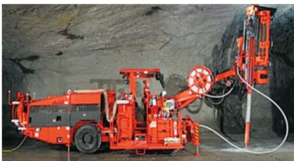
Figure 13. DD 420 providing the installation of cable-injection rods designed by Sandvik (Sweden), capacity – 50 thousand m/year
