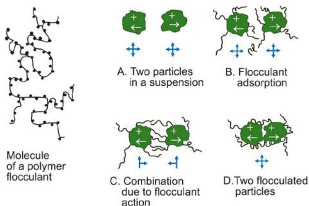
Figure 3. Formation of large floccules from flocculant monomers and tailing pulp sludge
