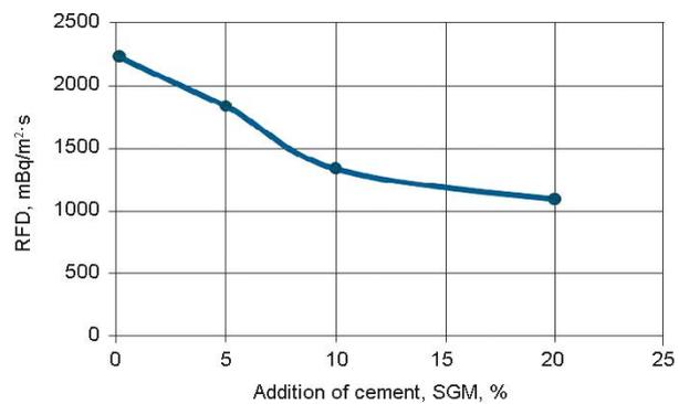
Figure 9. Changing radon flux density (RFD, mBq/m<sup>2</sup>·s) emitted by a paste based on materials from carbonate uranium ore processing depending on the amount of added cement (10%) and SGM (20%)
