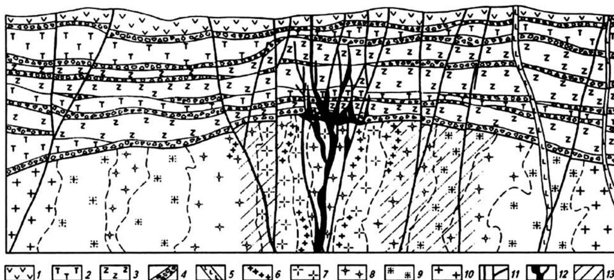
Figure 1. Geological section of the Streltsovskaya caldera: 1 – felsite; 2 – andesite-basalt; 3 – trachydacites; 4 – conglomerates, gravelstones, sandstones, 5 – mafic dikes, 6–10 – granitoids (6 – aplitoid, 7– pegmatoid, 8 – leucocratic, 9 – biotite, 10 – granite gneisses), 11 – faults, 12 – ore bodies, 13 – low uranium content areas
