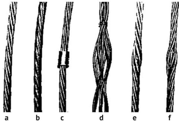
Figure 10. Types of cable rods: a – solid; b – with an epoxy envelope preventing corrosion under long-term operation conditions; c – with a steel clamp; d – with brace; e – with an insertable core; f - with a pear-shaped thickening
