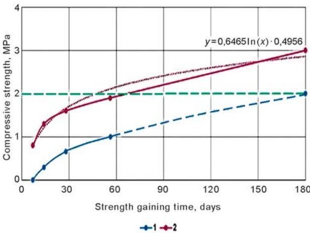
Figure 7. Compression strength (MPa) of paste samples based on uranium ore processing materials with an addition of cement (10%): 1 – carbonate ores, 2 – aluminosilicate ores
