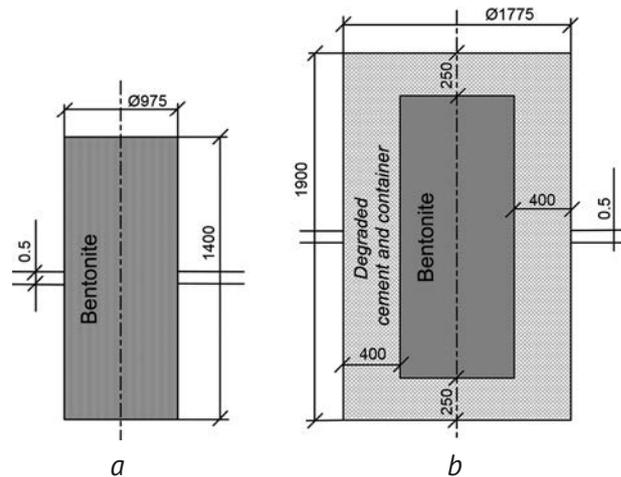
Figure 1. Bentonite cylinder crossed by a water-conducting fracture (a); bentonite cylinder in a permeable shell (b)
