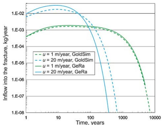
Figure 10. Comparison of calculation results for GeRa and GoldSim: impurity flows into the fracture given different GW rates for option B
