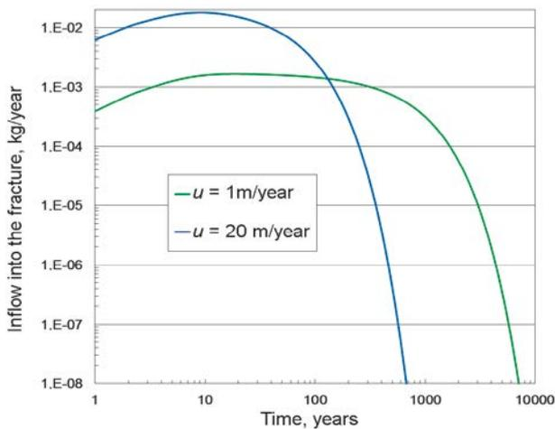
Figure 5. Conservative contaminant flow into a fracture crossing degraded backfill considering different groundwater flow rates (option B)
