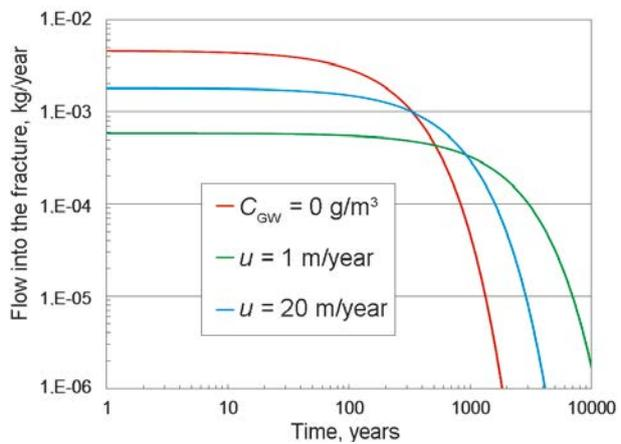
Figure 2. Conservative contaminant flow into a fracture crossing a borehole filled with bentonite considering different groundwater flow rates in the fracture (option A)
