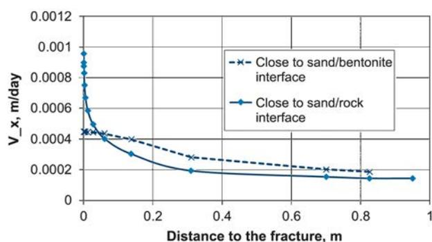
Figure 11. Dependence of the horizontal component constituting to the Darcy velocity in the backfill on the distance to the fracture plane (option B,  $u = 20$  m/year)
