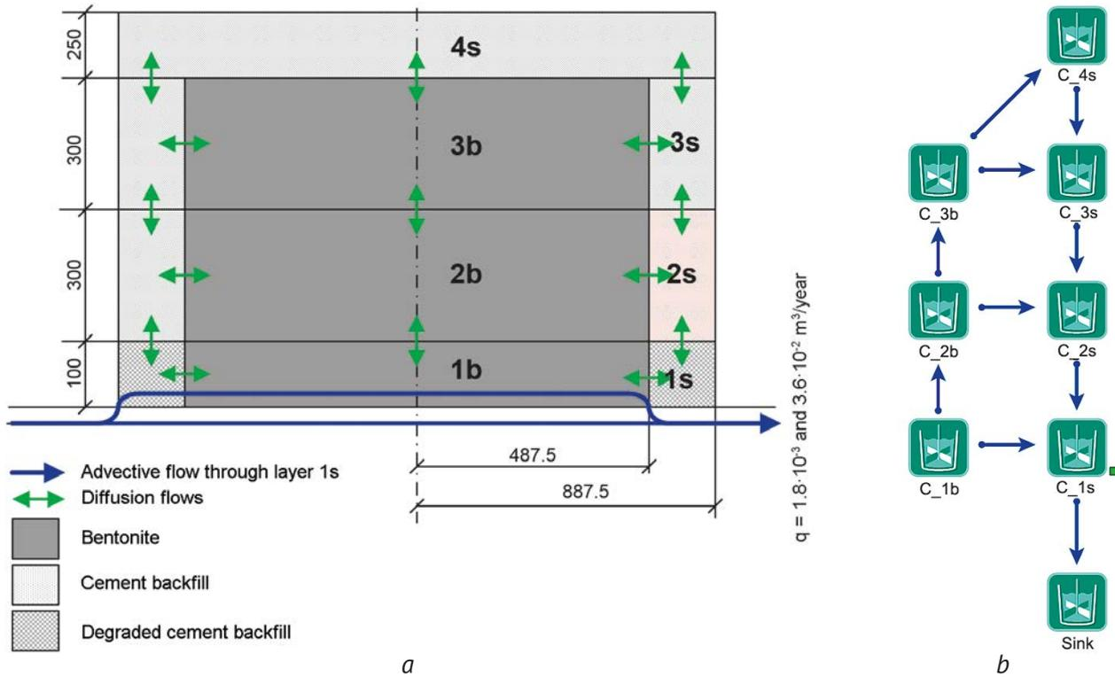
Figure 4. Geometry of a model with a degraded backfill adjacent to the fracture (a) and its representation in the form of "cell" elements in GoldSim (b)
