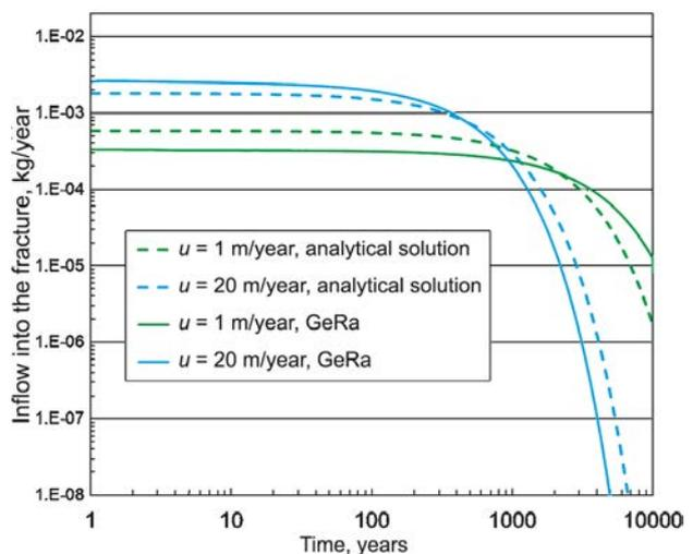
Figure 9. Results of calculations in GeRa in comparison with the analytical solution: contaminant flows into the fracture considering different GW flow rates for option A
