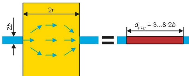
Figure 3. Equivalent volume model for a backfill capable of advective water transport
