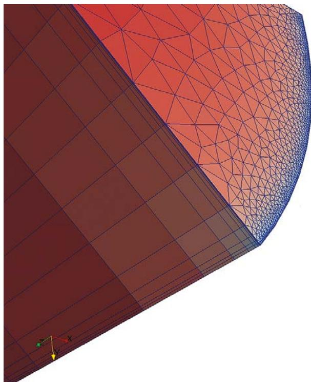
Figure 8. Partitioning the computational grid near the fracture boundary (partitioning fineness  $d=3$  mm)
