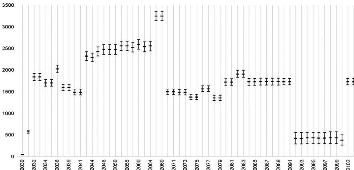
Figure 5. Expected load on the cementation unit by years (m<sup>3</sup>)
