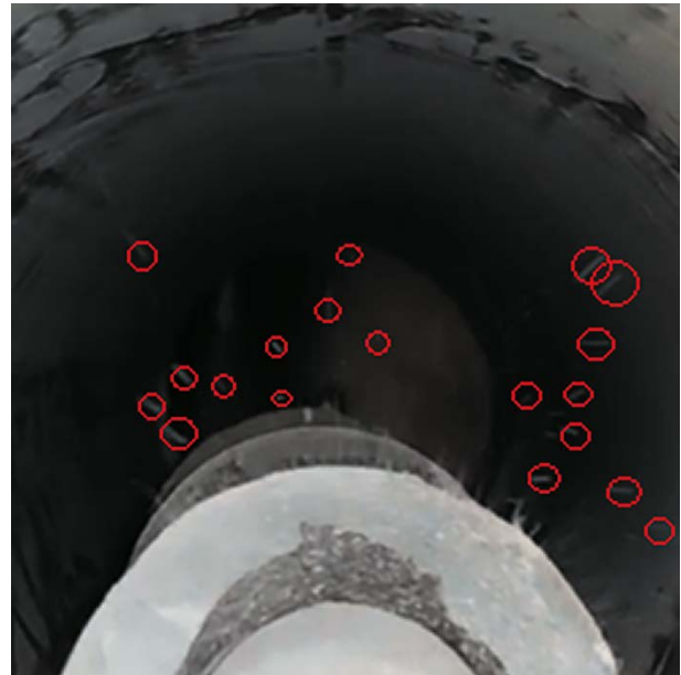
Figure 7. An example of a photograph that allowed to picture the suspensions discharged from the auger
