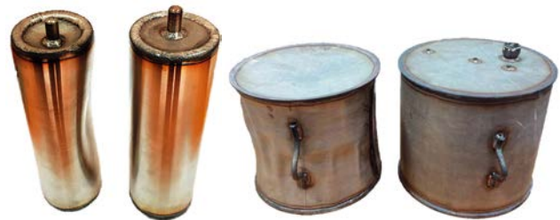
Figure 3. Changes in the metal capsule volume following HIP treatment
