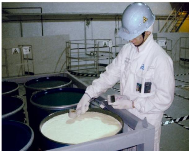
Figure 5. Radiation control of bottom residues processing products
