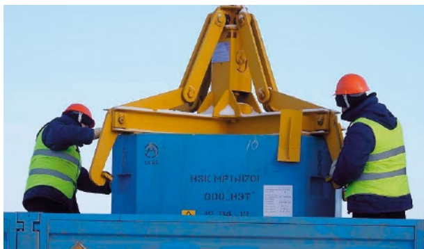
Fig. 1. Hooking RW package using a semi-automatic capturing device [4]
